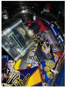
2) Remove old light bulbs and keep in mind where which color was. Slowly turn the old lampholder 180 degrees around, like in the picture. You may need a screwdriver to loosen this somewhat. Be very careful you don't short circuit any wires while turning the holders around. CHECK THIS VERY GOOD BEFORE GOING FURTHER!
