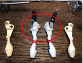
Slide the axis out and remove the broken bowling pin from the assy via removing a screw
