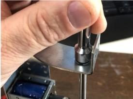
The ring has 4 'teeth' pointing inwards and upwards. The easiest way to slide it over the axis is have the 'teeth' pointing upwards to the end of axis
