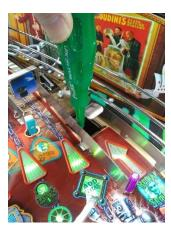
FORCE SCOOP TOP TO THE RIGHT BY PUSHING ON THE SCREW DRIVER (SCOOP WILL MOVE ABOUT ¼" or so)
