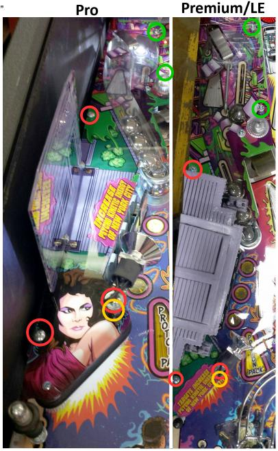
Flip Plastic #05 over in order to inspect the LED flasher PCB. The LED flasher PCB should have a non-conductive Mylar strip or fiche paper protecting the backside of the board.
