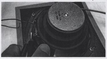
19) Use hammer and chisel to remove the wood woofer speaker mount. If you have a shaker motor installed, you may need to remove the shaker
