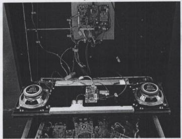
3) Remove the screw holding the cable clamp which secures the HDMI cable. Disconnect the DVI adapter from the monitor board.
