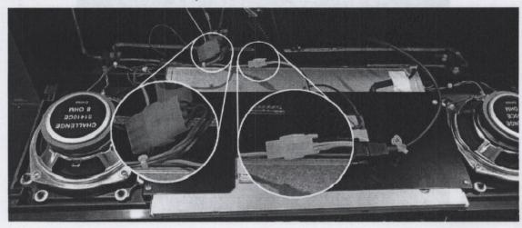
5) Remove old **On-Screen Display Keyboard**. There are two screws securing the board. Remove the cable connected to this as well. On different versions of Medieval Madness, this board is installed in different locations.
