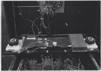
8) Connect the power cable that was disconnected from the old monitor to the new monitor.
