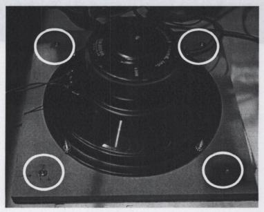
18) Cut the wires from the old woofer close to the speaker terminals.
