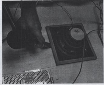
20) Once you get the chisel underneath the speaker spacer, you can start prying up. Note that here are four staples helping secure the spacer to the cabinet. The spacer can be removed by prying up from just the front side of the square.
