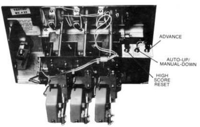
Figure 1. Door Diagnostic Switches
