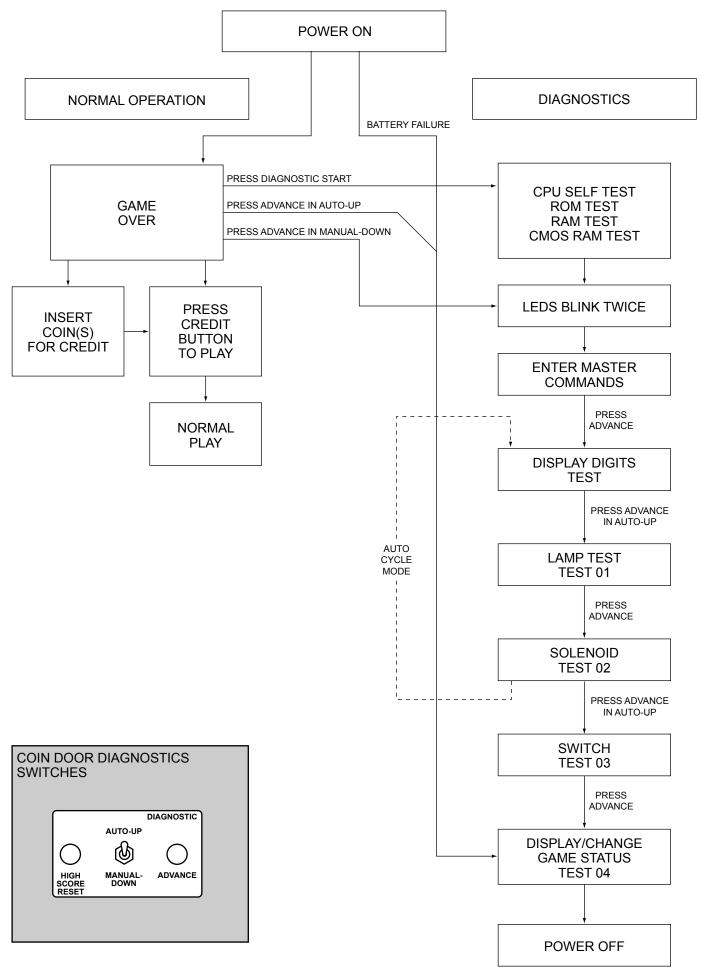
Figure 3. Normal Operation and Diagnostic Flow Chart
