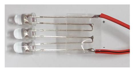
At 12 volts, 3 LEDs can be connected in series, with each of the longer (plus) and shorter (minus) leads of the LEDs connected. The minus pole of the 2 pin headers on the board is on the left side in the upper photo (marked with a black dot)
