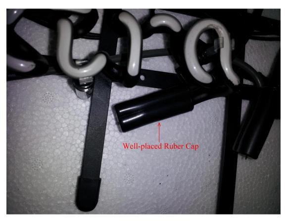
Step 8: Double check to make sure there is no exposed electrical wire. You are done! To test the sign, simply plug it in and cut it on.
