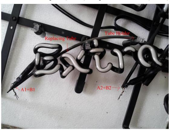
Step 5: Carefully set the tubing on top of each tube support. Adjust each tube support as needed to make sure lined up correctly.
