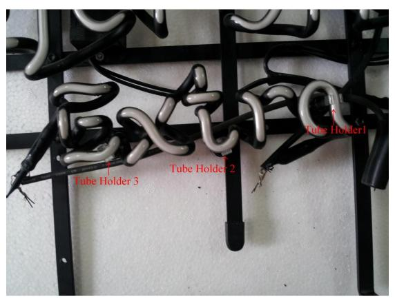
Step 7: Turn the twisted wire end backwards and replace the rubber end caps over the wire ends. Make sure the end caps are snug.
