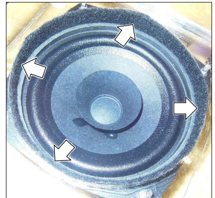
Fig. 2: Adhesive tape to prevent dazzle
