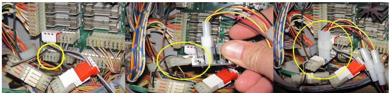
**8) Lower the playfield.** As you lower the playfield, there should be enough of a gap between the playfield backboard and the backboard artwork for the two harnesses. The lead coming off the back of the display should be long enough for the connector to pass beyond the backboard and not get pinched between the backboards.
