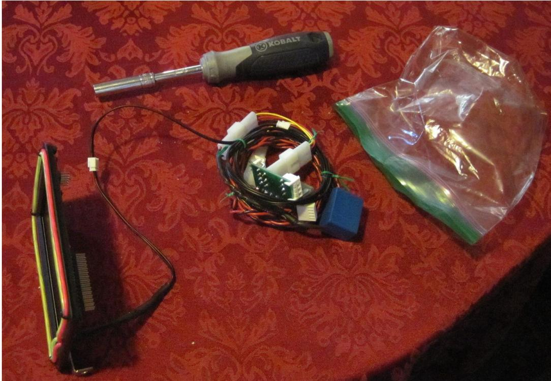
**4) Everything should be plugged together except the white square connector on the red/black harness. You can place the Power Tap and harnesses over the back of the playfield and into the cabinet for now, but hang on to the white square connector on the red/black harness.**
