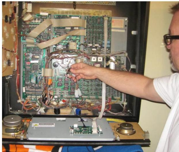
**7) Find J117 on the driver board (lower left corner). Unplug the connector at J117 and plug it into the male pins on the Power Tap before mounting the tap to the driver board. Plug the Power Tap into J117. Be sure you have the tap aligned on the pins properly.**
