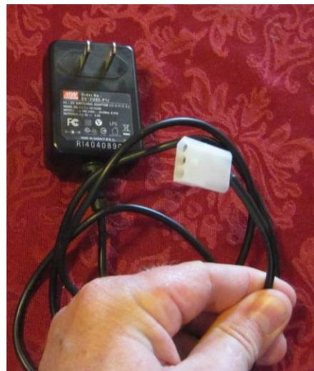
Please be aware of how this standard 3-pin is set up. Sending improper voltage to a mod could result in damage to the mod.
