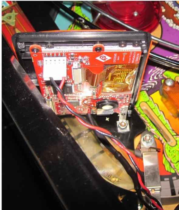
**6) From the right side of the cabinet, swing open the backglass light board. Reach into the back of the cabinet and grab the power tap. Lower the speaker panel and feed the Power Tap under the backboard artwork and up through the head.**
