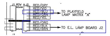
Note: The interface of Row#6 to the EL LAMP Board is not mentioned in the BBB schematics
