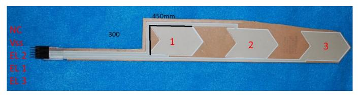
Wire the EL arrow with the identically labeled connections of the "EL" header on the EL board. It does not matter which of the 3 Vss pins is used – they all offer the same EL operating voltage.
