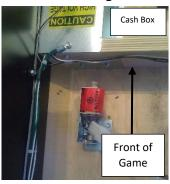
4) Center the Knocker Coil on the Strike Plate, the Front Part of the Metal Bracket Needs to be 1 3/16 away from the Knocker Plate, Fasten with 3 of the ½" Screws.
