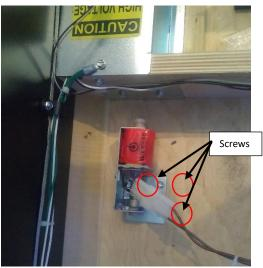
5) Connect the small 3 pin connector to DRV-5 on the ADD ON BOARD, then connect the other end to the Knocker Coil - #A. (The ADD ON BOARD is on the inside left wall of the cabinet farthest from the front)
