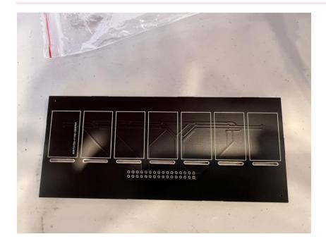
Install the 16 way 2 pin right angled header. NOTE: this goes on the FRONT facing side of the PCB, NOT the side with the pre-soldered FPC Sockets.
