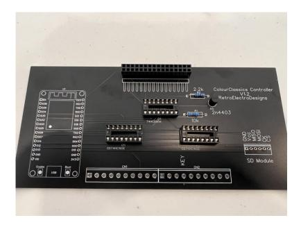
Install the 2 single pin 15w female headers for the ESP32s board:
