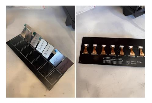
Once all screens have been tested and are working ok, secure to the PCB with either glue or double sided tape. Use the thinnest double-sided tape you can get.
