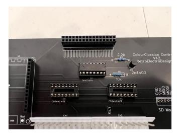
Install the 2 X "165" IC's in to the left and right sockets:
