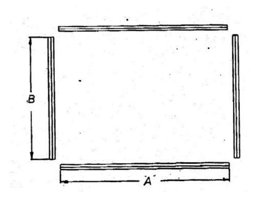
A = the length of the top or bottom of the translite/Backglass + 1/16" – (less) the thickness of one board B = the length of the sides of the translite/Backglass + 1/16" + the thickness of one of the board
