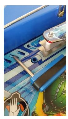
**(2)** Push fit a stainless steel sleeve supplied into each blue nylon flipper bush from the top of the playfield, initially by hand. You should be able to easily push them in more than halfway. Take care as the ends are sharp!
