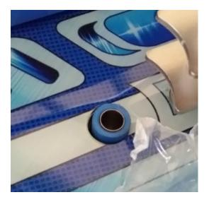
**(4)** Look carefully on the under side of the bush to see if any swarf has been pushed out of the nylon bush. If so, remove it.
