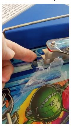
**(3)** Using the insertion tool supplied, use a small hammer to GENTLY tap the bush home. It should be installed all the way, the tool will 'bottom out' and rest flush with the top of the nylon bush.
