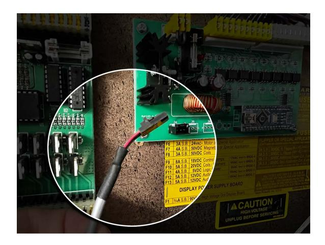
You're ready to connect to the topper. First step is take the long grey cable and plug one end of it into the new circuit board, down in the lower left corner.
