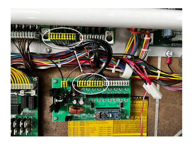
Plug one yellow connector into the place you just removed the white connector from.
