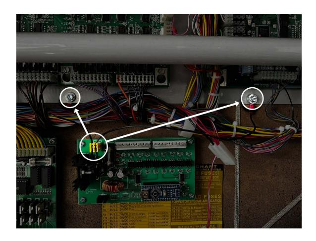
Plug the yellow connector with two wires coming off of it into the upper left of the new circut board.
