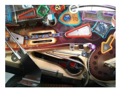
11. REPLACE THE 1/4" SCREW CLOSEST TO THE POST, MAKE SURE THE BALL GUIDE IS TOUCHING THIS POST. CAREFULLY APPLY PRESSURE TO THE BALL GUIDE SO YOU CAN REPLACE THE SECOND 1/4" SCREW FROM THE RIGHT AND TRY TO STRAIGHTEN OUT THE BEND BEFORE FULLY TIGHTENING THE SECOND SCREW. NOW REPLACE THE THIRD 1/4" SCREW, YOU MIGHT HAVE TO APPLY PRESSURE ON THE BALL GUIDE TO LINE UP THE SCREW HOLE. THE FINAL GOAL IS TO HAVE THE BALL GUIDE TOUCHING THE POST ABOVE THE MILK CAN LOOP.
