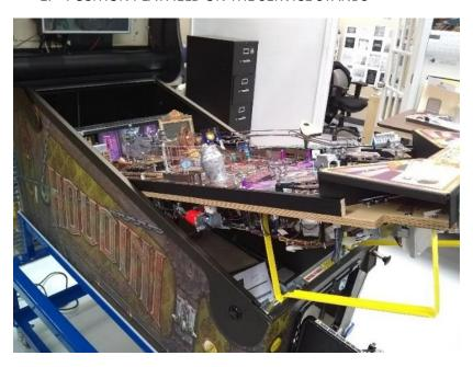
2. REMOVE THIS UPPER PIECE OF PLASTIC BY LOOSENING THE 2 PHILLIP SCREWS.
