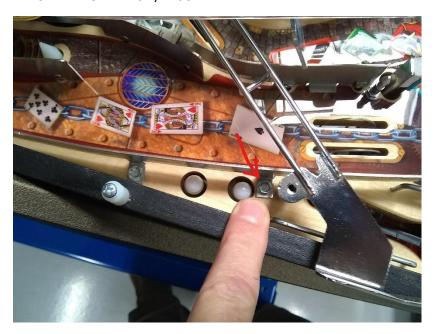
9. CAREFULLY LIFT UP ON THE METAL BALL GUIDE AND MOVE TOWARDS THE CENTER OF THE PLAYFIELD
