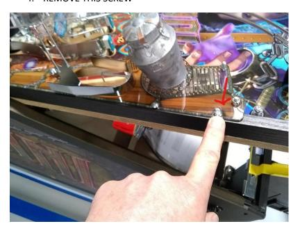
5. LOOSEN THIS SCREW AND REMOVE 2 – 11/32 ACORN NUTS CIRCLED.
