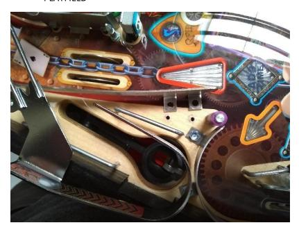
10. BEND THE BALL GUIDE JUST NEXT TO THE LEFT MOUNTING TAB, BEND IS EXAGGERATED FOR THE PICTURE.
