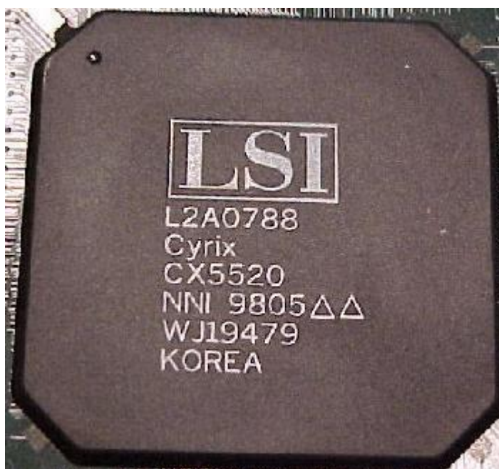
The Cyrix 5520 companion chip used in the Pinball 2000 motherboard.
