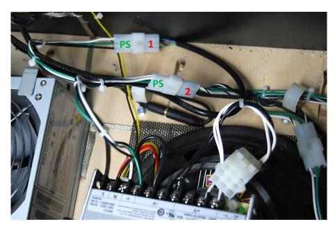
Using a  $\frac{1}{2}$ " magnetic nutdriver and two #8 x  $\frac{1}{2}$ " SMSs  $\frac{44}{2}$ , attach the new power supply (by way of the two L brackets you installed earlier) to the bottom and back wall (or just the back wall) of the lower cabinet (mark and predrill pilot holes).
