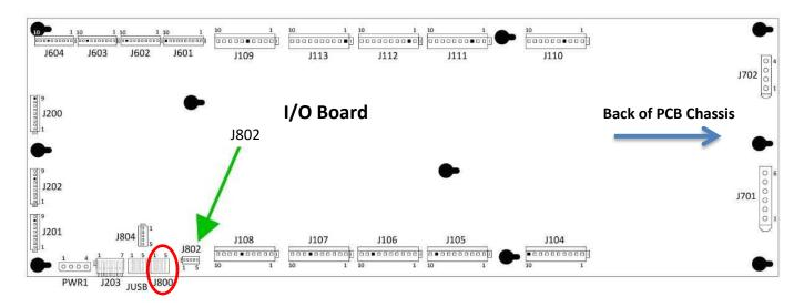
Locate the USB cable connected to J800 (circled in red above) on the I/O bd. Follow one of the two steps below:
