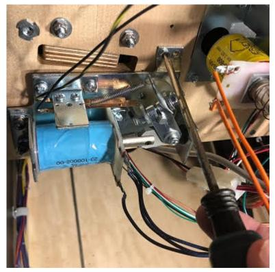
Carefully lift it down off of the playfield. The slot is slightly shorter than the diverter flag - yours may be missing so what I am saying here may only apply when you go to re-install the mech. - so you have to angle it a bit to get it out of the hole:
