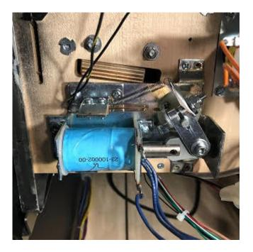
Note that I have already removed 5 of the six mounting screws in the above picture. You need a #2 philips or a 1/4" nutdriver to remove them, and remember that once you start loosening the last one, the mechanism will want to fall down so make sure that you hold it.
