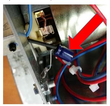
**Step 2**: Completely clip off the capacitor at its base on both sides to remove it from the motor assembly. Do not clip the blue wire on accident.
