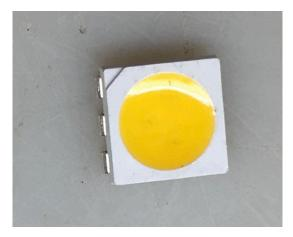
3. Solder a 150  $\Omega$  resistor to the SMD's observing polarities (notches). Solder wire to the other side of SMD's. See sketch above for notch locations.
