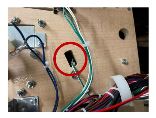
11. Trace wires from sensors back to four-pin connector marked "orange" and remove old sensor assembly
