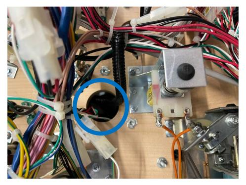
9. Carefully unclip zip ties to free wires
