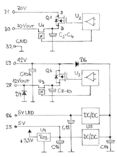
Note: I saw some melted 70V MOSFETs (see pictures above). The reason is unclear to me and I ask myself, if a simple fuse could not replace those switches...
