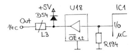
Note: Typically there should be a resistor between an output and the first controlled LED (on the playfield boards? check). But the ferrite [L3] might also do the job (resistance?).
