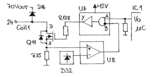
Note: The over current protection is disabled for all MOSFETs on current I/O boards by replacing all measuring resistors with 0 Ohm devices and additionally shorting them with a common wire. Obviously this circuitry caused problems, the additional wires could be an indication of some oscillation tendency.
