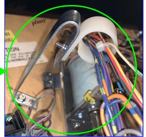
Four of the wiring harness standoffs were too tall after installing the new Stern style playfield support brackets and needed to be lowered.
