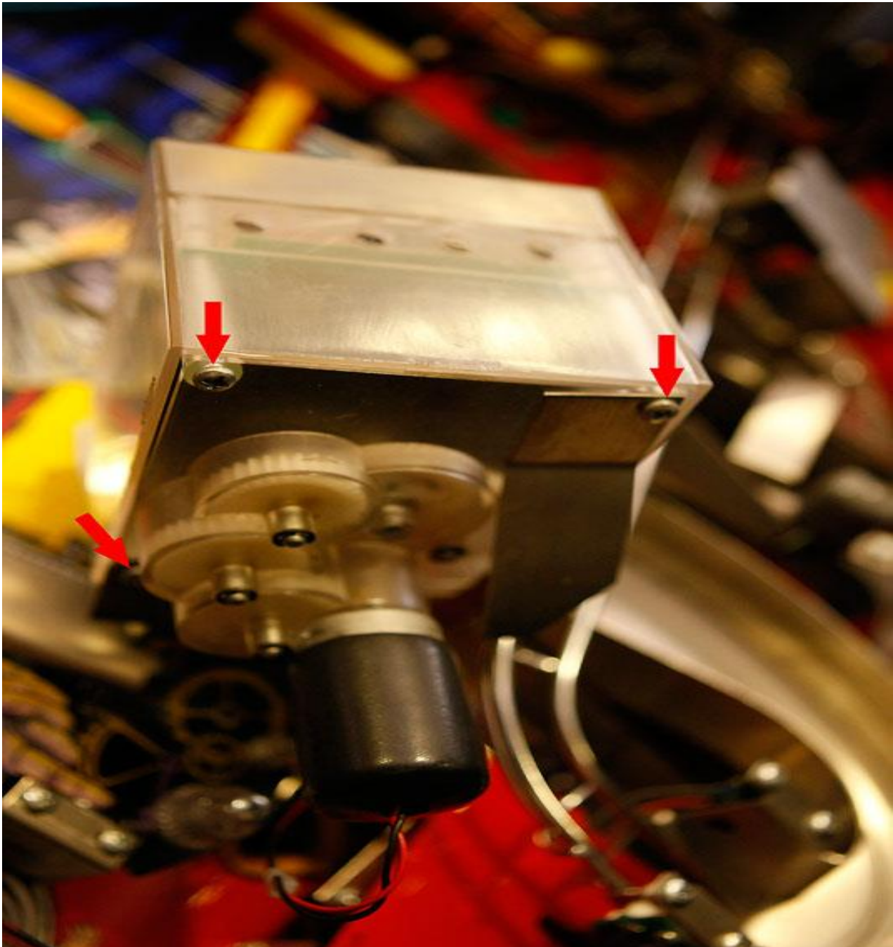
Image 4: 3 of the 4 back screws (the 4th is behind the bracket in this photo)
