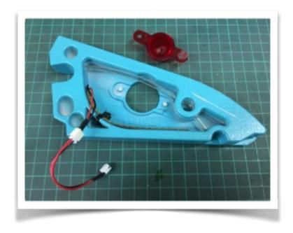
Then locate the Clamp Plate into the mod - note: before installing you first need to tap the hole in the centre hole refer to Section 3.
