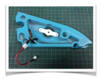
Then for the v2.0 owners place a small dab of hot glue over each locator pin to lock in place. This is done mainly so when you loosely install the signage you can swing it out of the way making the installation of the mod back into the game easier and then swing the sign into the preferred position and nip up the centre screw knowing that the Clamp Plate will not drop out mid way through the install. The photo shows V2.0 owners what the small dabs of hot glue will look like.
