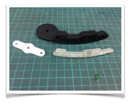
Clamp Plate - you need to tap a thread into the hole in the centre of your white Clamp Plate, this could be done with a tap or force cutting by winding either 4mm bolt or equivalent imperial bolt through the hole.
