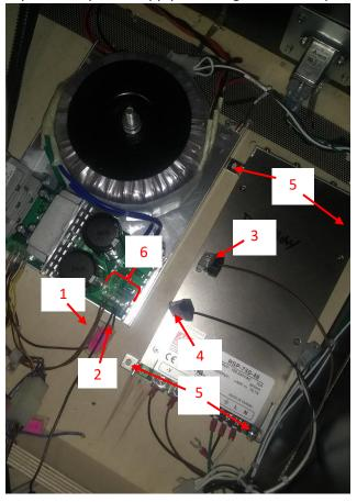
Remove the 2 Brown wires from the old P.S. #1, ensure there is a half inch of insulation removed from the wire and insert into an empty slot on the brown Wall Nut #3. (your game may have more than 2 Brown Wires, attach all of them to the Brown Wall Nut #3)
