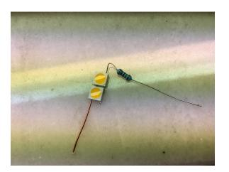
5. Insert resistor through hole and solder. Solder other wire (copper wire in picture) to lamp base, then clip excess wires.
