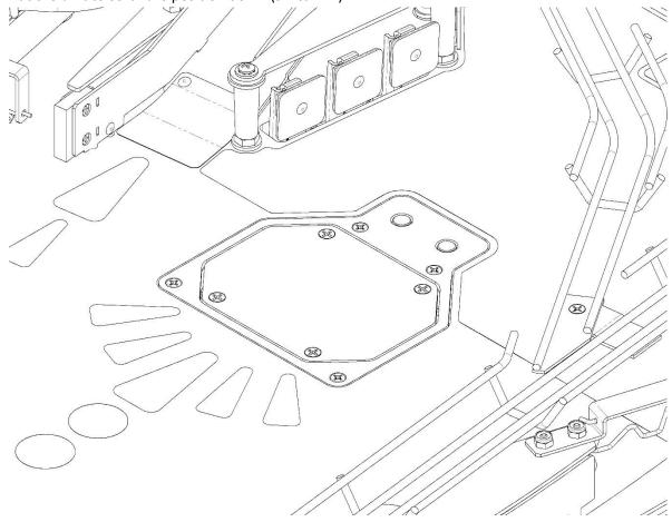
2. Using the 5/16 nut driver, loosen the 3 nuts on the bottom stop bracket (front side of unit). The bracket should be now resting on the single adjustment screw.
