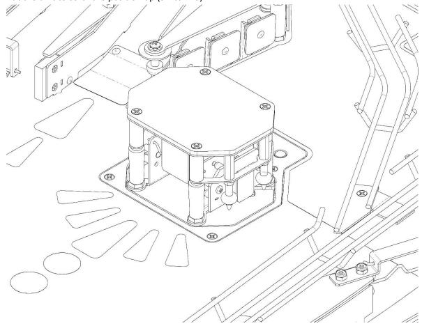
2. Using the 5/16 nut driver, loosen the 3 nuts on the motor mounting bracket (back side of unit). The bracket should be now resting on the 2 adjustment screws.
