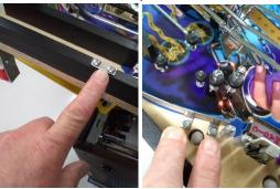
Remove the flat rail and open the radius of the curve about 1 inch.
