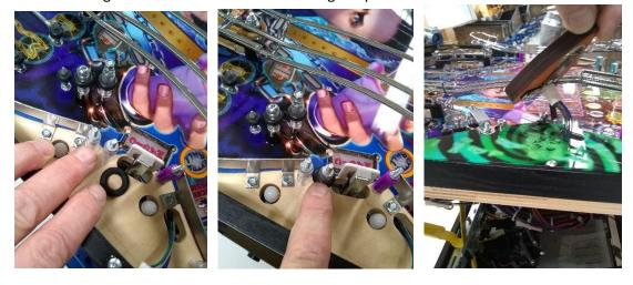
Reinstall the gate, plastic and planchet. Test to ensure the ability to hit all three stand up targets from the shooter lane.
