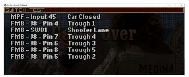
If you have doubts about a certain switch, you can check the correct working here. Push the switches on the MPF (parking targets, loop ramp, ramp made, closed door) and see if this switch pops up on the display here. Check that the 2 parking targets are not always lit (which means a stuck switch) Also, a sound can be heard when a switch is activated and you can also see if there are no switches active when they should not be.
