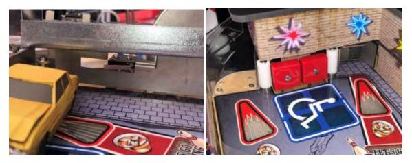
So if the cardoor swings open and is stutters against the parking targets it means the parking switches are not triggered and need some re-adjusting. If it doesn't close properly the Close switch needs readjusting.
