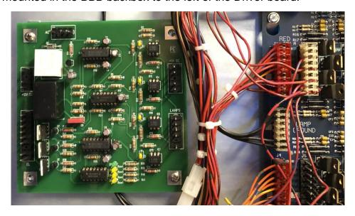
The next sections describe a step-by-step startup procedure by gradually connecting the 5 Molex headers on the board shown in the picture below. The pin assignment is identical to the CAPCOM board. Therefore, original cables can be used and the board can be exchanged 1:1.
