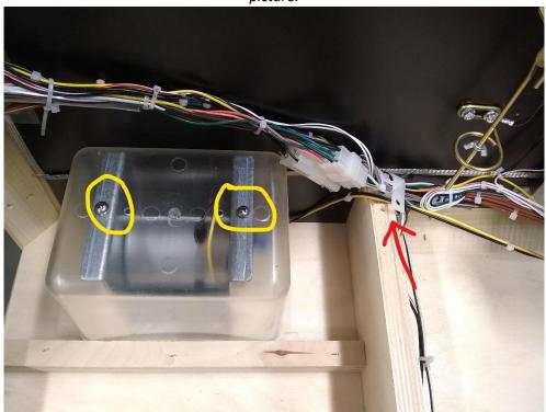
Route the shaker motor cable and plug into the ADD ON BOARD to DRV 2. See picture
