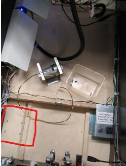
Turn game off remove glass and lift the playfield all the way up so it is leaning against the Backbox. Position shaker motor over mounting holes with wires orientated to the rear of the game. *See picture.*
