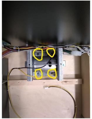
Install shaker motor cover with the remaining screws <u>be mindful that the cable is not in the path of the</u> <u>spinning weight.</u> Then remove wire keeper and route shaker motor cable under it and replace screw. *See picture.*
