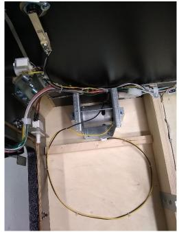
Using the 4 like screws fasten the shaker motor to the pinball. See picture.
