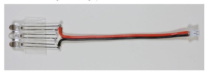
A hidden and well protected (!) location for one LED group is located between the plastics behind the front left ramp. I've cut a foam block to fit and provided holes for the LEDs (the picture shows an resistor in the lead during my tests).
