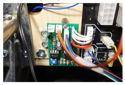
Remove the original Xeno Drive connector carefully (!) and plug it into the Flasher board (K1), which in turn is connected to the Xeno Drive header.
