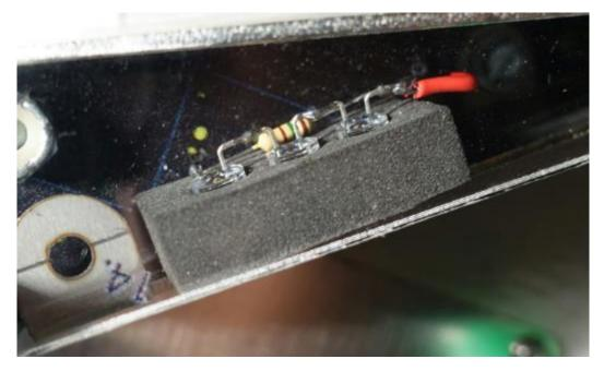
A second piece of foam with corresponding recesses forms the rear end, the whole construction is then clamped together between the plastics.
