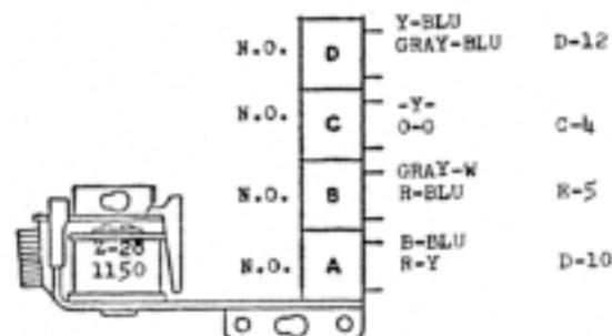
IN SERIES WITH SWITCH C-19 ON 3-IN-LINE RELAY.
