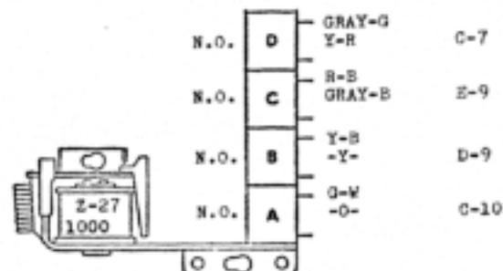
IN CIRCUIT TO BALL COUNT RESET COIL AND GAME-OVER RELAY TRIP AND LATCH COILS.
