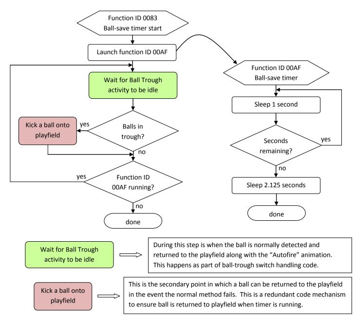
As shown in the logic flowcharts, above, there are 2 separate functions that are running for auto-fire timer:
