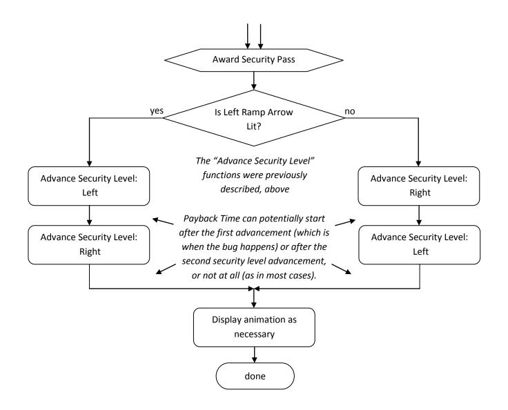
The flowchart for the "Award Security Pass" function is depicted above. This function simply checks if left ramp arrow is lit and uses it to decide whether to advance the security levels in the order of left then right or in the order of right then left. After advancing the security levels, there is some logic to determine whether to display an animation before finishing.
