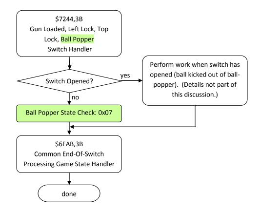
The simplified flowchart, above, shows how the ball-popper handler, when switch is closed (ball landed on ball popper switch), performs a state check 0x07 (details further below) followed by a \$6FAB,3B end of switch processing. This end-of-switch processing is actually called from a variety of sources as depicted below. This common function then spawns a separate function to perform further work as described below.
