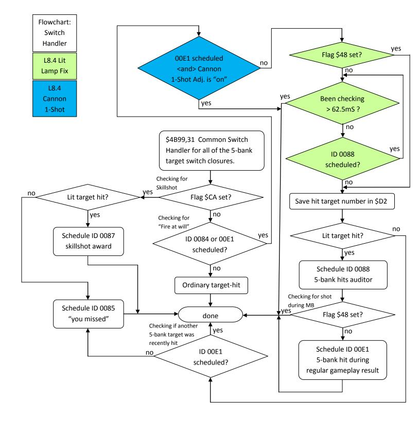
The logic for limiting each cannon shot to a single target hit is highlighted in the blue addition to the switch handler flowchart, above.
