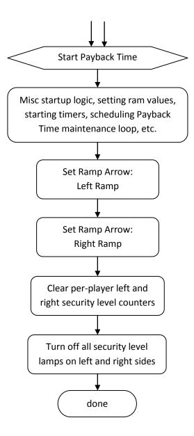
The "Start Payback Time" function, as depicted in the flowchart above, performs some basic housekeeping and schedules a separate function to maintain the Payback Time state. The housekeeping, as shown, includes specifically setting the left and right ramp red arrows as well as extinguishes the left and right security level lamps.
