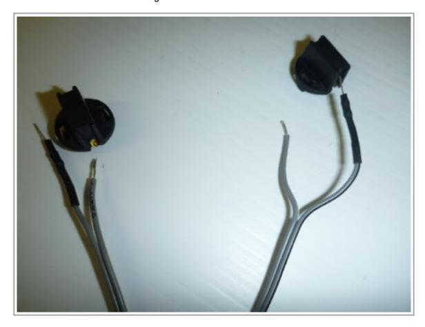
• Install a led and plug the red wire into the "Parking Ok" and the white led into the "Move Your Car.
