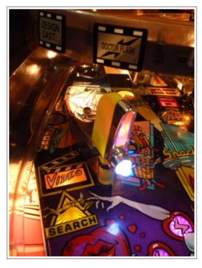
of the cable tie moved a little and when the target was hit next to the mod it got stuck in as got caught up with the target. You will see the target get caught and held back and your game will get a error dot with the error on the cola target.
