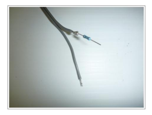
• Now cut 1 x piece of 2.5mm heat shrink as well as a 50mm of about 5mm heat shrink and slide of the cables and then solder the 2 x positive leads from the leds to the resistor, and repeat for the negative leads.
