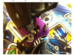
2. Insert both sets of wires on the new cabinet through the playfield hole and seat the base on the two screw posts. Replace the hex screws and slide the zip tie back on. Reattach the bounce protector *in reverse*, with the curved side facing away from the mini-cabinet.
