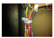
the way down the playfield, using zip ties as necessary, and up the large hole in the rear to the back box. Remember to leave enough slack to account for a fully raised playfield. Remove the backglass
