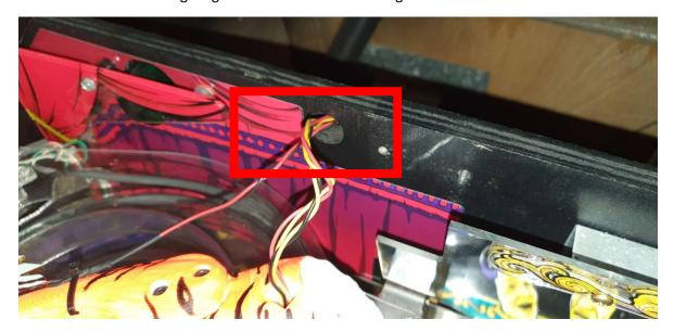
5. Use right hole to feed mounting screw (M5) through backboard.
