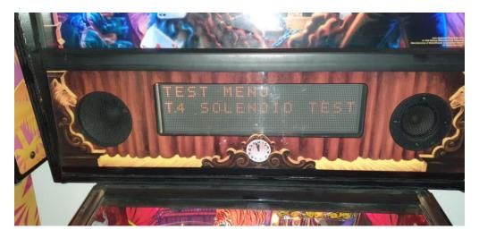
4. Go to T.4 19 Tiger Saw Motor when it is on repeat saw blade will move a bit and eyes will lit
