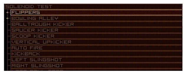
With the + - buttons, you can select the coil you want to test. Go down and select left and right ball gate and run a test via pushing Enter button when ball gate is selected
