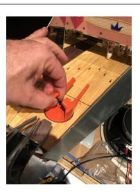
The 2.5 mm Allen screw to tighten the launcher is found at the right and best approachable when the launcher is positioned like in the above picture
