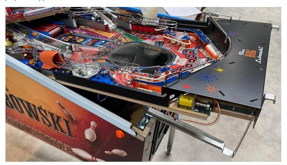
In this position already the ball trough can be observed and checked if connectors are properly in place. Otherwise proceed to step 2 in required
